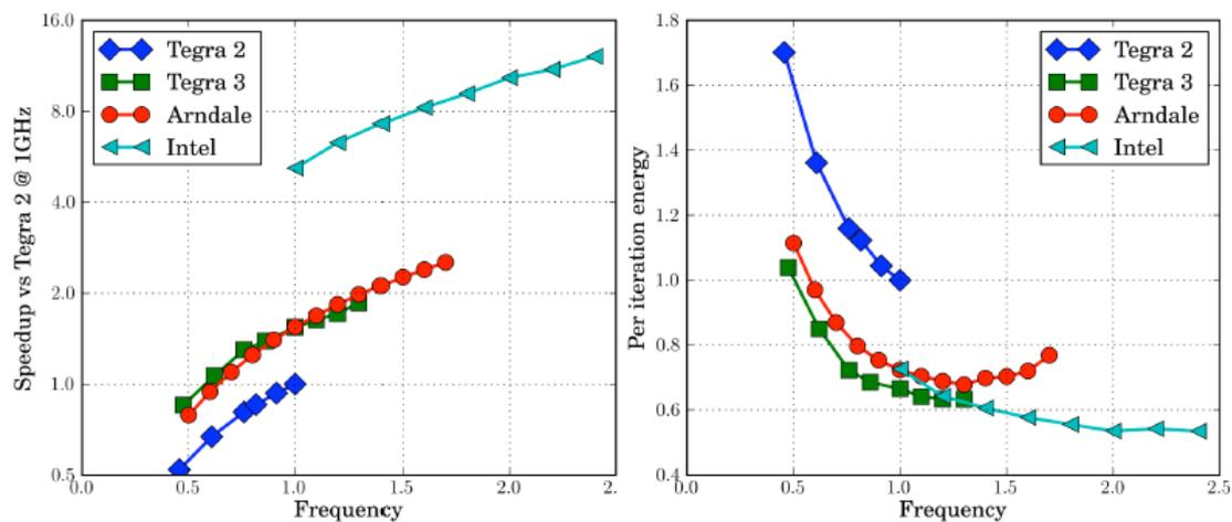
**Figure 3 - Multicore performance and energy of Arndale boards (dual-core ARM Cortex- A15) against Tegra2 (dual-core ARM Cortex-A9), Tegra 3 (quad-core ARM Cortex-A9) or Intel x86 Core i7 (quad-core Sandybridge at 2.4 GHz)**
