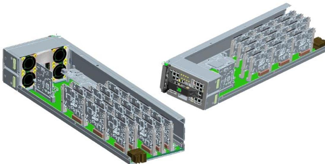
**Figure 2 - Picture of a Mont-Blanc blade fitted into BULL standard format**
