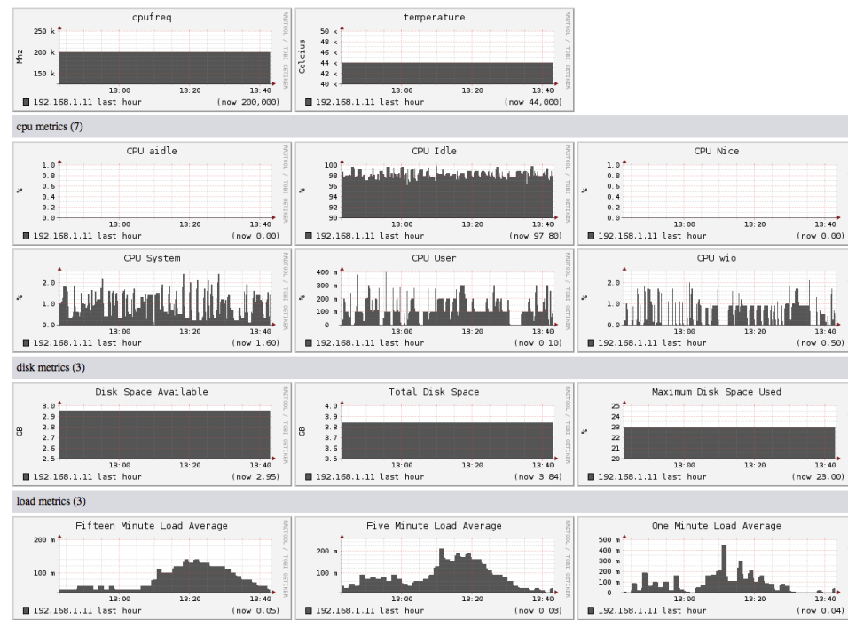
Figure 1: Example output from the Ganglia web-front end monitoring a single Arndaleboard
